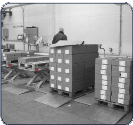
Low profile lifting tables can easily be set up as part of a packing line.
