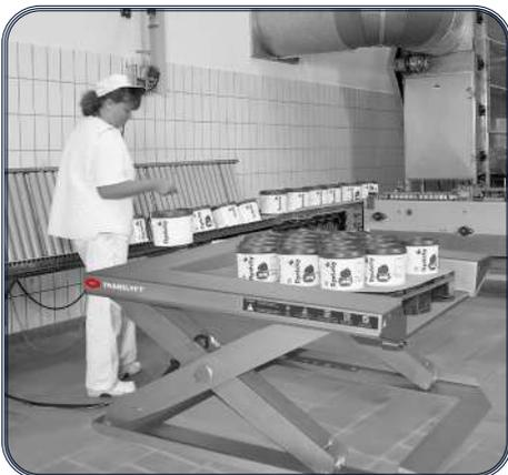
The stainless steel solution makes it perfect for rugged conditions and the use of aggressive cleaning products like in the food industry.
