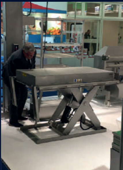
4: Put table in cleaning position
