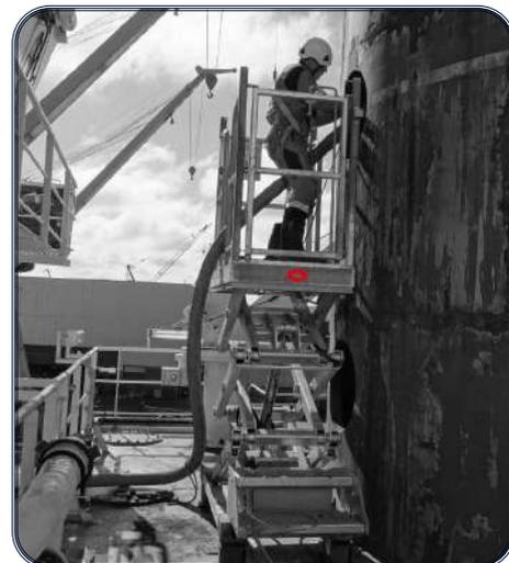
All lifts can be produced in a painted steel, stainless steel, galvanized steel or a solution with a mix of the three.
