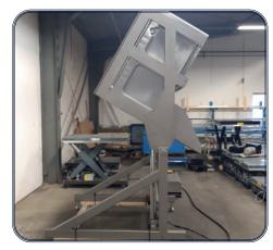
The 120 degreee tilt function easily tilts the content onto the next process point of your workflow.
